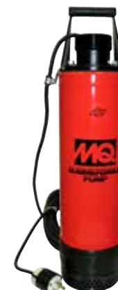
The pump model ST3020BCUL provides its own internal thermal overload protection, however, the 230V 1Ø CB6 Control Box is offered for convenient ON/OFF/AUTO and float switch operations. The CB6 comes standard with two SW1WOPA float switches.
